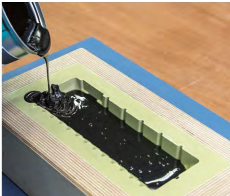
Casting of foundry pattern out of EPO 5019
