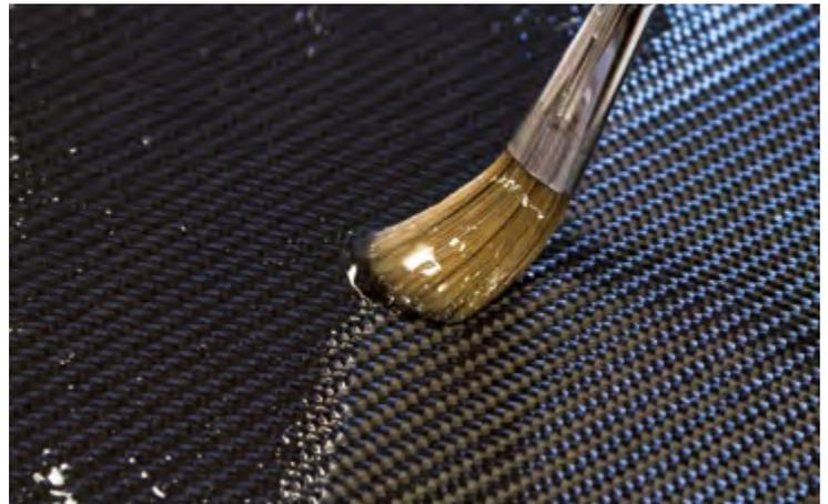
Biresin® CR82 with optimized viscosity for wet lay-up
