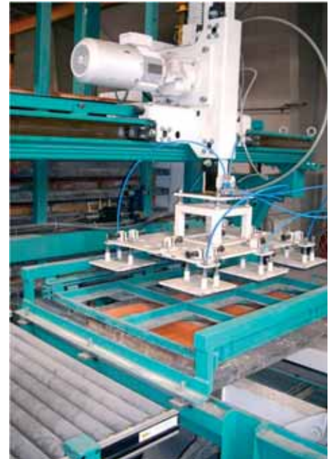
Automatic demoulding Equipment (vacuum lifting).
