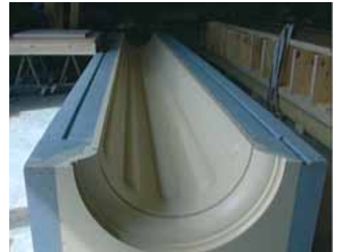
UR 5830 Mould of column for 10 shots only.
