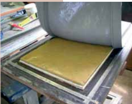
UR 5863 MOULD making over F18 fastcast master mould.
